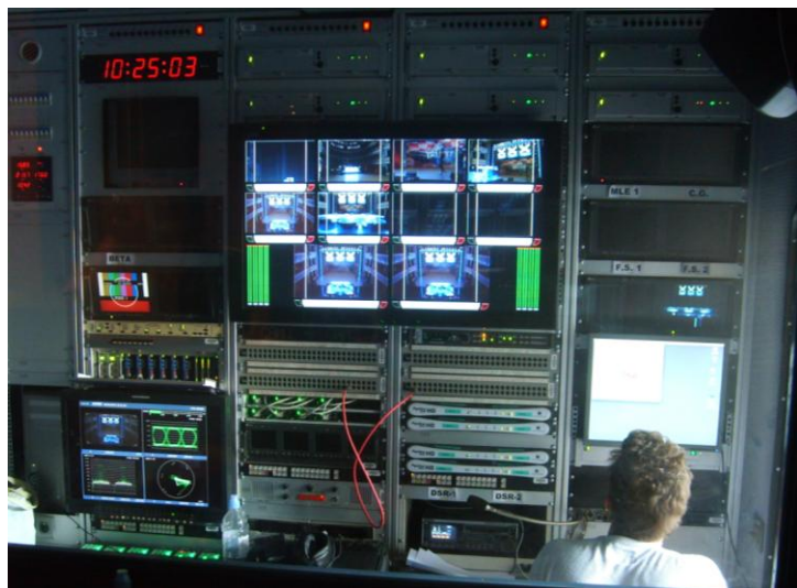
Telestream Pipeline HD Dual systems installed in Nova TV HD-OB van.
